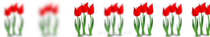
The camera may move the focus motor in the wrong direction first, and may pass through proper focus as it searches for optimal contrast.
